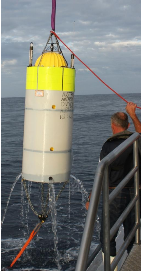
Figure 12 Recovery of the prototype acoustic mooring trialled during the March voyage.
